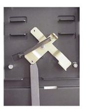
**Unlocking from the bottom**: Slide the tool in from the bottom, keeping the open side of the hook to the left, as shown. Catch the lock and pull down.
